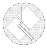
I Place the two pieces of card edge to edge and mark a line for the Depth Allowance on both pieces of card.
