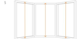
Measure the drop from where the top of the blind will sit to where you want the blind to end. This is the DROP measurement.
